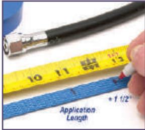
Measure the sleeving and mark the measurement with a pen or marker. Add an additional 38mm-51mm and cut the extended length of sleeving.
