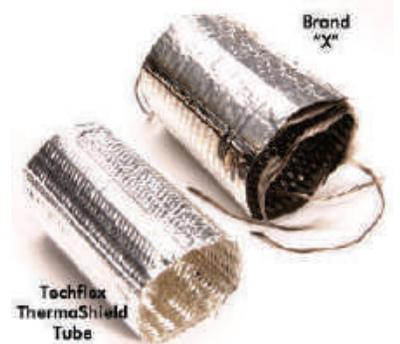
Techflex ThermaShield and a competitor's similar product were placed in the same electrical test oven for one hour at 626°F (330°C). Note the burning and delamination of the fiberglass interior of the Brand "X" product. Even the metallic shroud suffered a degree of burning and brittleness that did not occur on the ThermaShield sample.
