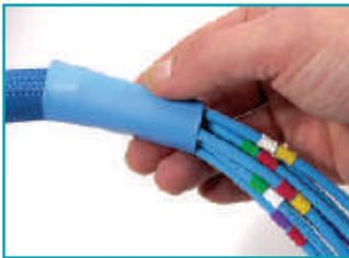
Slip the tubing over the bundle and position it so that both the sleeved and unsleeved portions are sufficiently covered. Notice the small pieces of tubing installed on single wires as part of a color coding system. If your project requires multiple operations, always work up from the smallest to the largest bundle.
