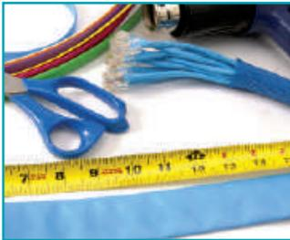
Measure the heatshrink tubing to length and cut with a scissor. The thickness of your bundle, as well as the desired final appearance, will determine the length of the tubing you cut. Generally, a piece 1 1/2" - 2" long will accommodate almost any need (such as this bundle of network cables). Single wires, or smaller bundles, require shorter pieces.
