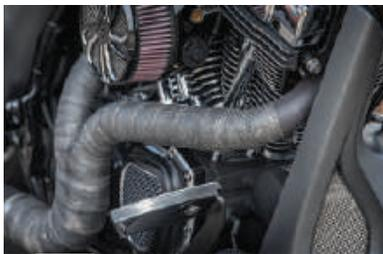
HEADER WRAP INSULTHERM™ (HFN) is extremely resistant to high temperatures. It is commonly used for automotive and high performance headers and exhausts.
