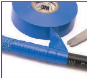
Starting at the line, take a few tight turns of tape down the application so that it covers the sleeving and extends about 38mm on the application. Make sure the tape is smooth and tight. Cut the end and press down for a smooth finish.
