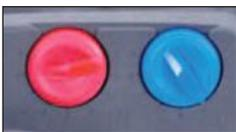
Adjustable heating power continuously by potentiometer.
